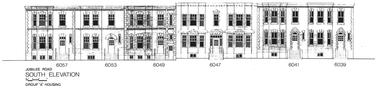
Figure 4: Edward Maxwell's rowhouse development. 6047 Jubilee Road is the only timber-frame building and it is twice as wide as the other rowhouses constructed of load-bearing brick.
