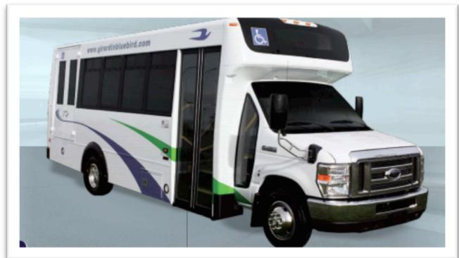
A typical minibus is a body build where a cabin body is fabricated onto a truck chassis. The body-on-chassis approach gives the advantage of higher seating capacity, or more room for passenger comfort through a larger cabin area. There is also the advantage of
