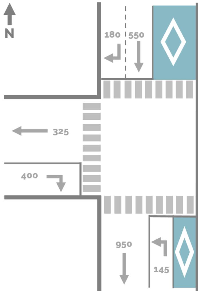
In the example shown on the left (the numbers represent hourly volumes), the NBT delay would not be included in the car delay average weighing since cars are prohibited on that movement. All other movements would be included in the calculation. Where cars are permitted on all turning movements, the overall intersection delay can be used. Therefore, this measure can be equivalent to the intersection delay measure for trucks.
