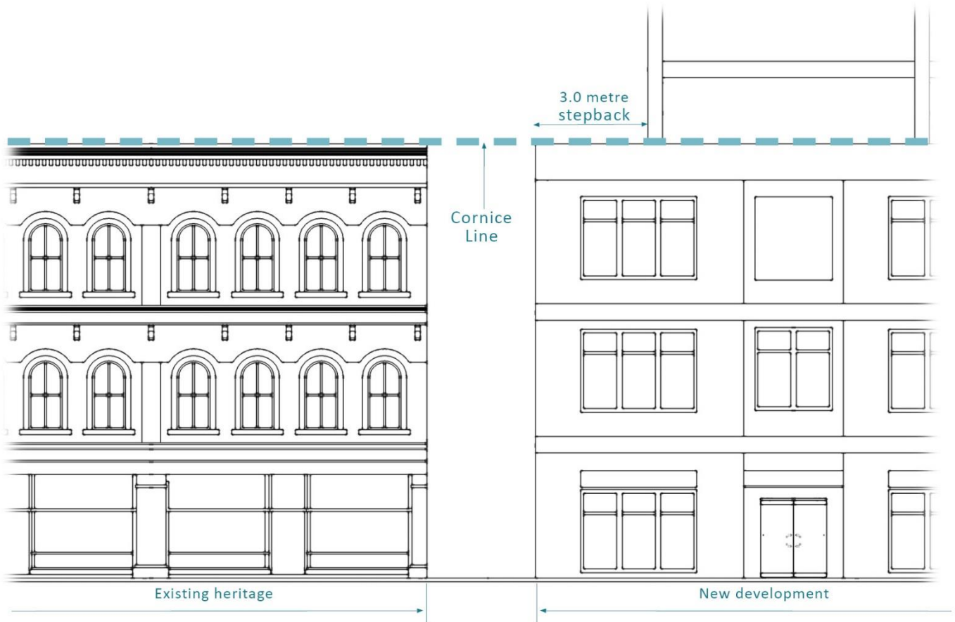
Diagram 15: Side wall stepback for taller portions of new detached buildings in a heritage context, as per Section 149
