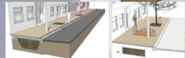
**3** Continuous soil trenches with paving bridges, structural soil or planting cells help to ensure the health of trees in tight spaces.
