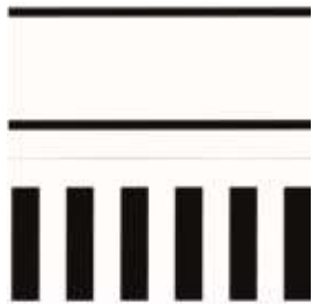
Parallel and Zebra Crosswalk Markings (NSTIR)
