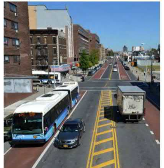
Figure 7: Separate Bus Transit Lanes Carrying BRT Services (New York City)
