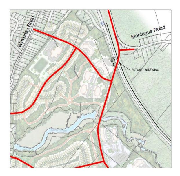
The challenge with crossing Highway 107 at this location is the angle of crossing and the proximity to the Montague Road interchange. The proposed bridge would cross Highway 107 at an approximate 40-degree angle which would increase the span length. The on and off ramps to the Montague Road interchange would also need to be accommodated making the total span of roughly 60 metres.
