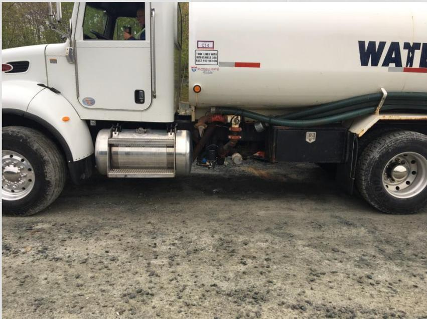
Fuel Tank & Intake/Discharge
