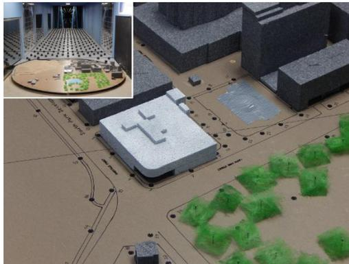
**Image 1: Wind tunnel model of the existing site and surroundings in 2015**
