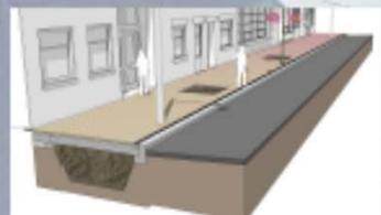
**3** Continuous soil trenches with paving bridges, structural soil or planting cells help to ensure the health of trees in tight spaces.
