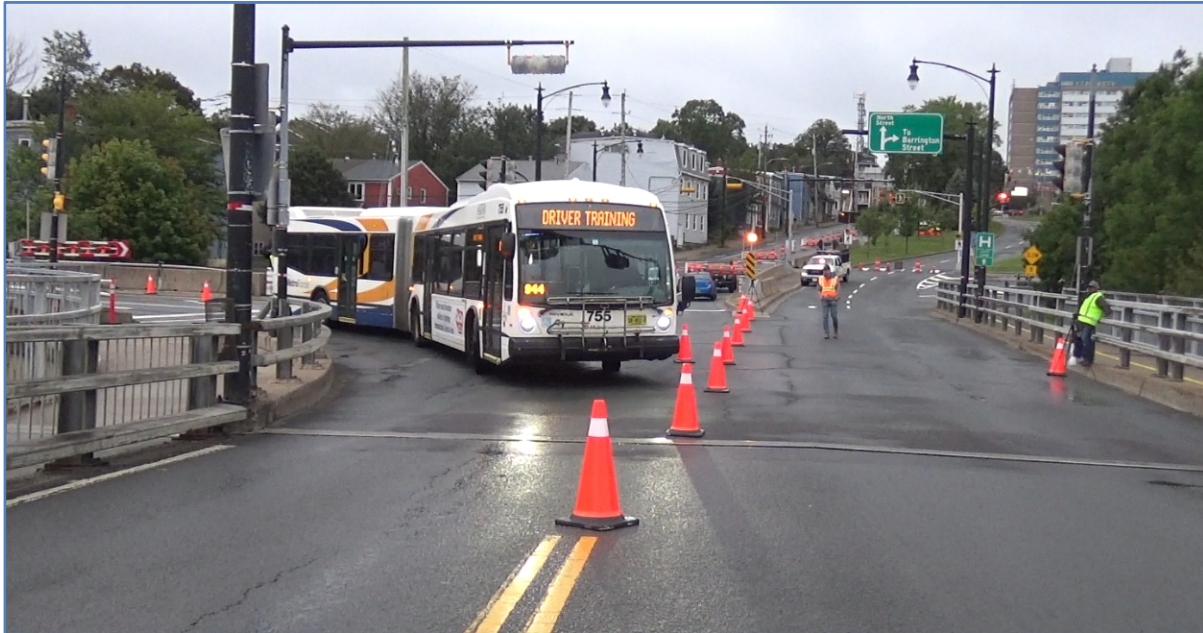
Figure 13 Successful Turning Movement of Articulated 60 foot bus into the Bridge Right Lane, Using the Modified Inside Lane
