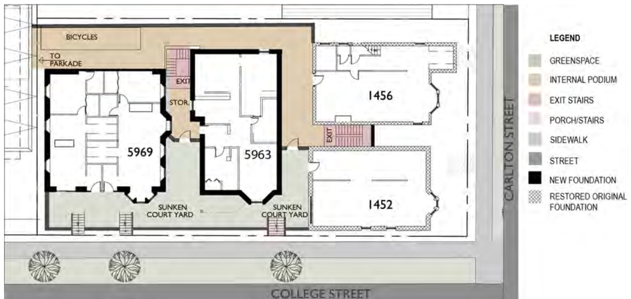
Figure 5. Proposed modification to 5659 College St., 5963 College St., 1452 & 1456 Carlton St. at basement level, by Architect.
