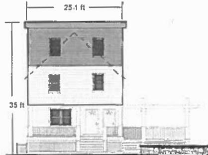
*Fig. 2: Dashed red line shows existing roofline, shaded blue area shows proposed change.*
