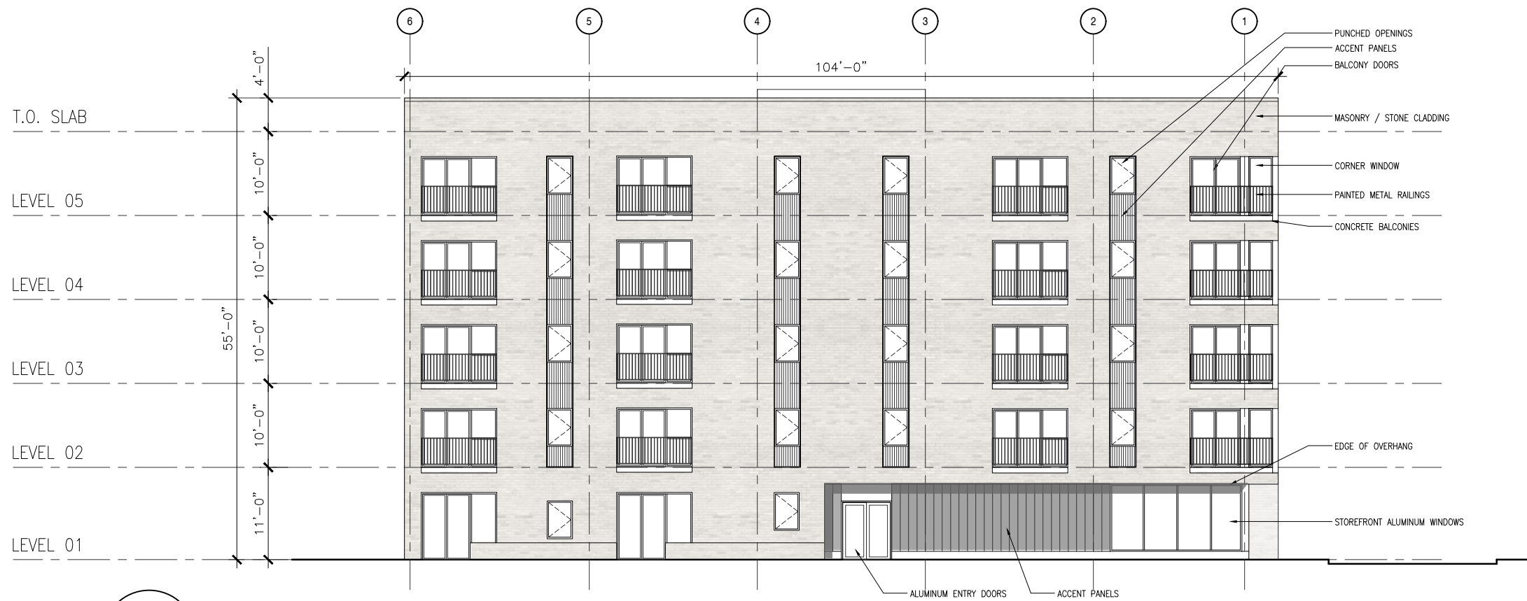
1/16"=1'-0" 1 BUILDING ELEVATION - FRONT
