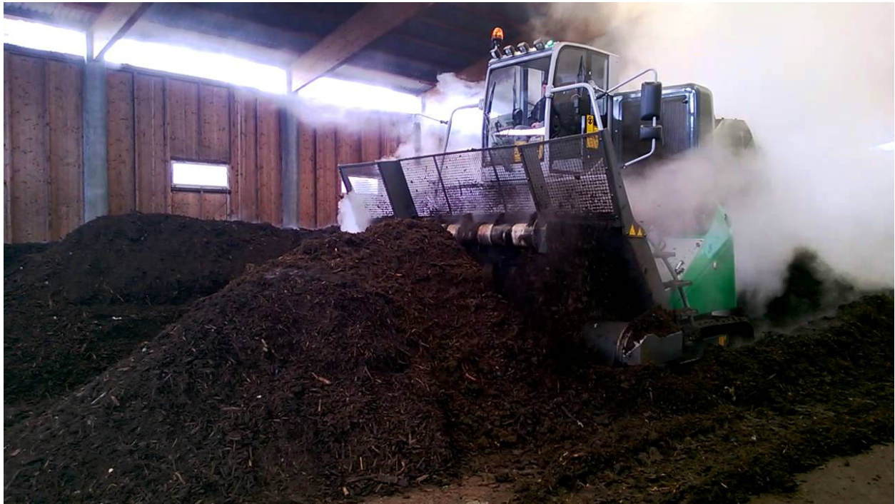
Figure 0.2: Photo of neuson-ecotec ECO 5003 (Source: neuson-ecotec website)
