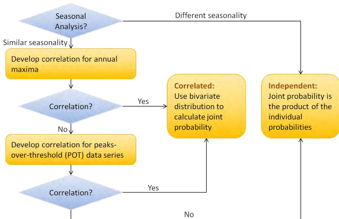
Figure 2.13 Flowchart for Determining Level of Correlation
