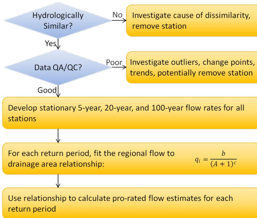
Figure 2.12 Flow Chart for Flow Pro-rating Analysis
