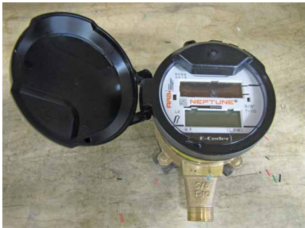
Typical 5/8 inch (15 mm) residential water meter
