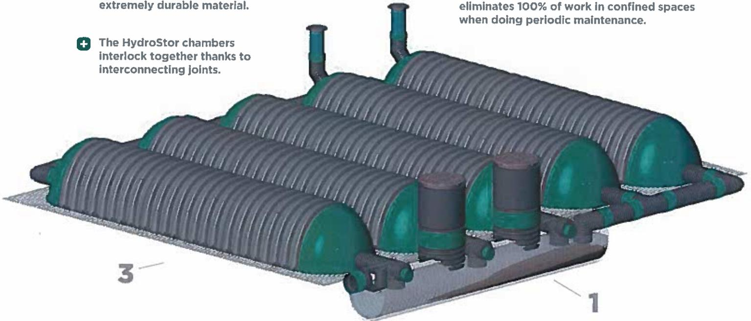
**1** The HydroStor pretreatment unit which is included in the system upstream of the diffuser eliminates the possibility of sediment migration to the chambers. Fine particles, obeying the Stokes law\*, remain trapped there. With its unique design, the system prevents the dispersion of hydrocarbons and floating debris.
