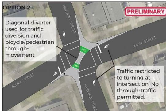
Figure 4: Plan View of Diagonal Diverter
