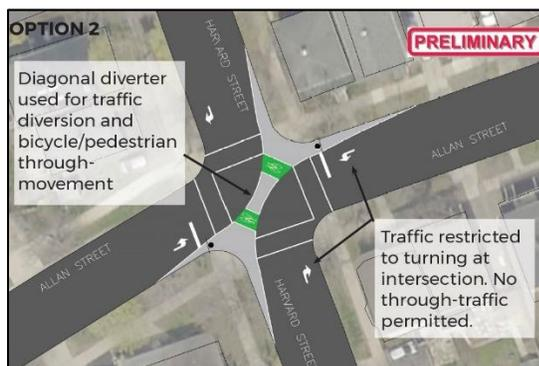
Figure 6: Plan View of Diagonal Diverter
