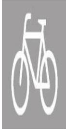
The bicycle symbol indicates that this section of the roadway is part of a bicycle lane. They are designed to advise motorists that an area of the street has been set aside for bicycles and that cyclists are present in the area. The symbols are designed to indicate to cyclists the location of the bike lane.
