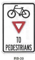
Figure 11: Cyclists yield to pedestrians sign (Source: Bikeway Traffic Control Guidelines for Canada, Transportation Association of Canada)
