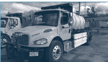
This truck has a sideguard installed. Sideguards save lives, and are being installed on all HRM and contractor vehicles over the next three years.
