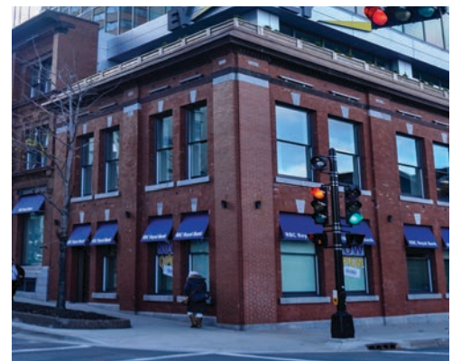
Figure 80. Awnings and canopies shall respect the edges of facade features such as windows.
