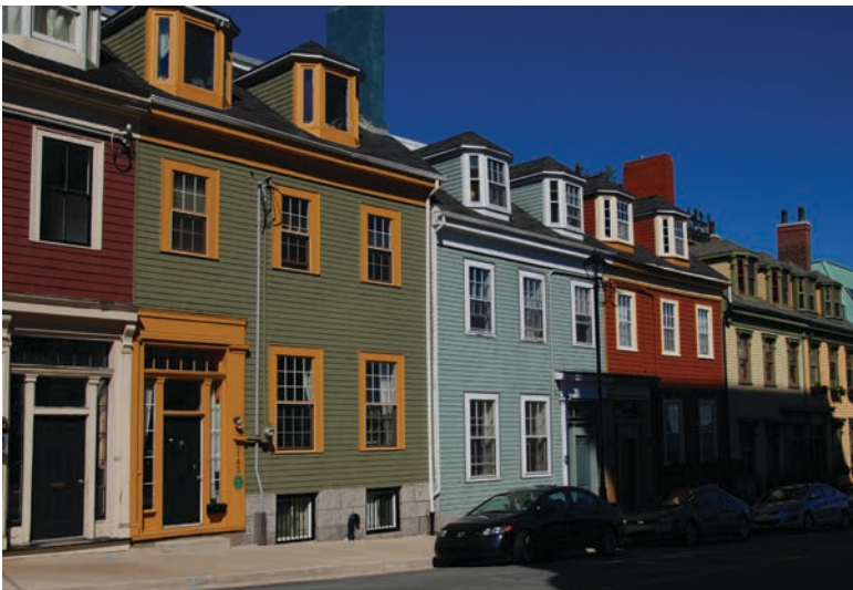
Figure 61. A heritage colour palette is selected for the row of houses, and the painting scheme highlights the articulation of the heritage resource.
