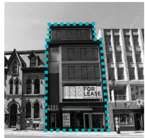
Figure 66. An example of new development infilling between heritage resources--the new structure is a significantly different style, but respects the spatial relationships and scale of the adjacent heritage structure
