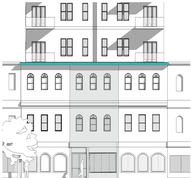
Figure 65. The cornice line is consistent between new development and the abutting heritage structures
