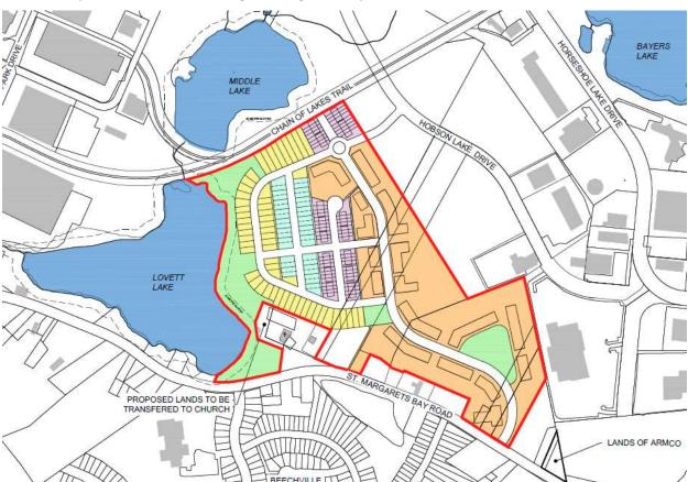
The proposed concept provides two access points to the development: one via St. Margarets Bay Road and the second to the future Hobson Lake Drive in Armco's Bayers Lake Phase 5.
