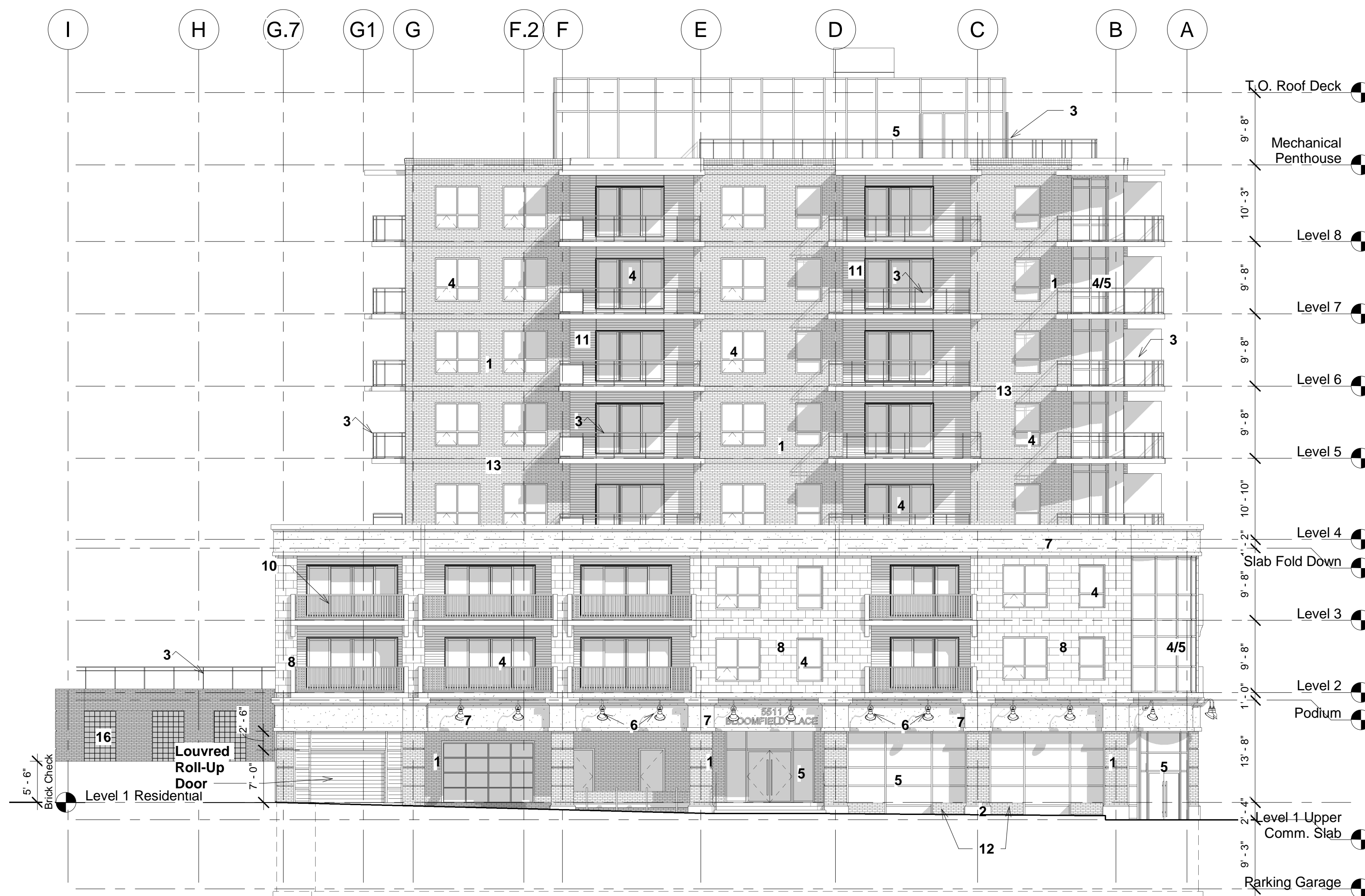
① South Elevation DA 3/32" = 1'-0"
