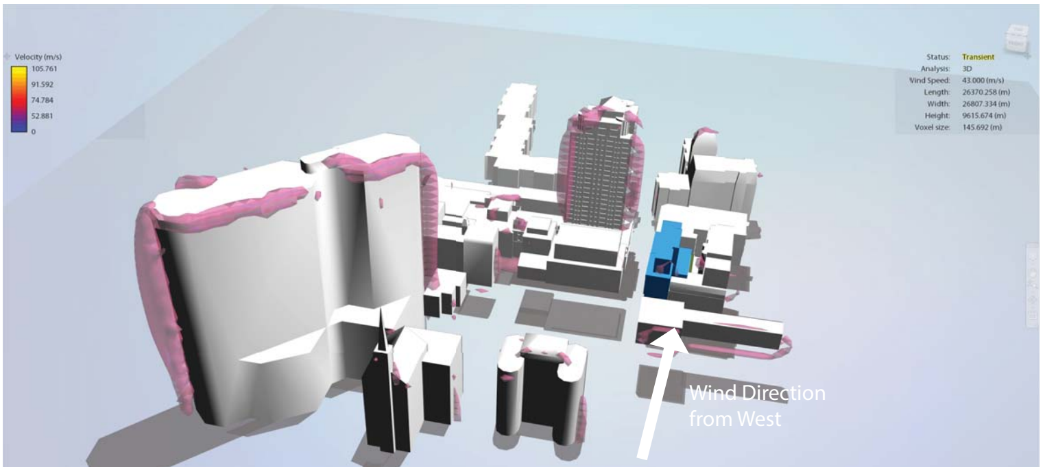
Fig 8. Westerley wind direction iso-surfaces. This purple surface shows a 70m/s wind zone resulting from a starting wind speed of 30 m/s.
